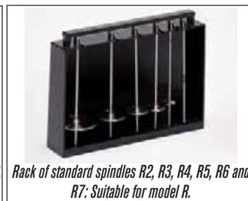
Rack of standard spindles R2, R3, R4, R5, R6 and R7: Suitable for model R.
